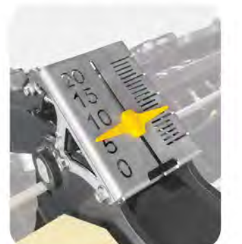
Graduated roller adjustment scale / Scaletta registro rullo
