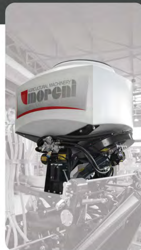
Pressurized seed hopper with hydraulic fan / Tramoggia in pressione con ventola idraulica
